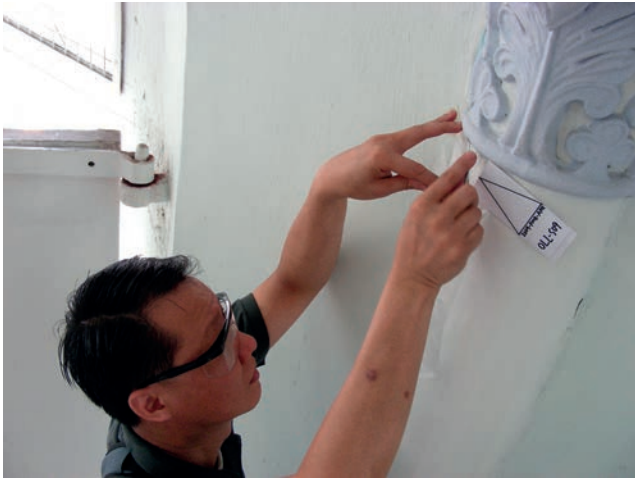
Figure 7 Paint sampling at the Church of Our Lady of Lourdes, April 2009. (Photo: Claire Lim)
