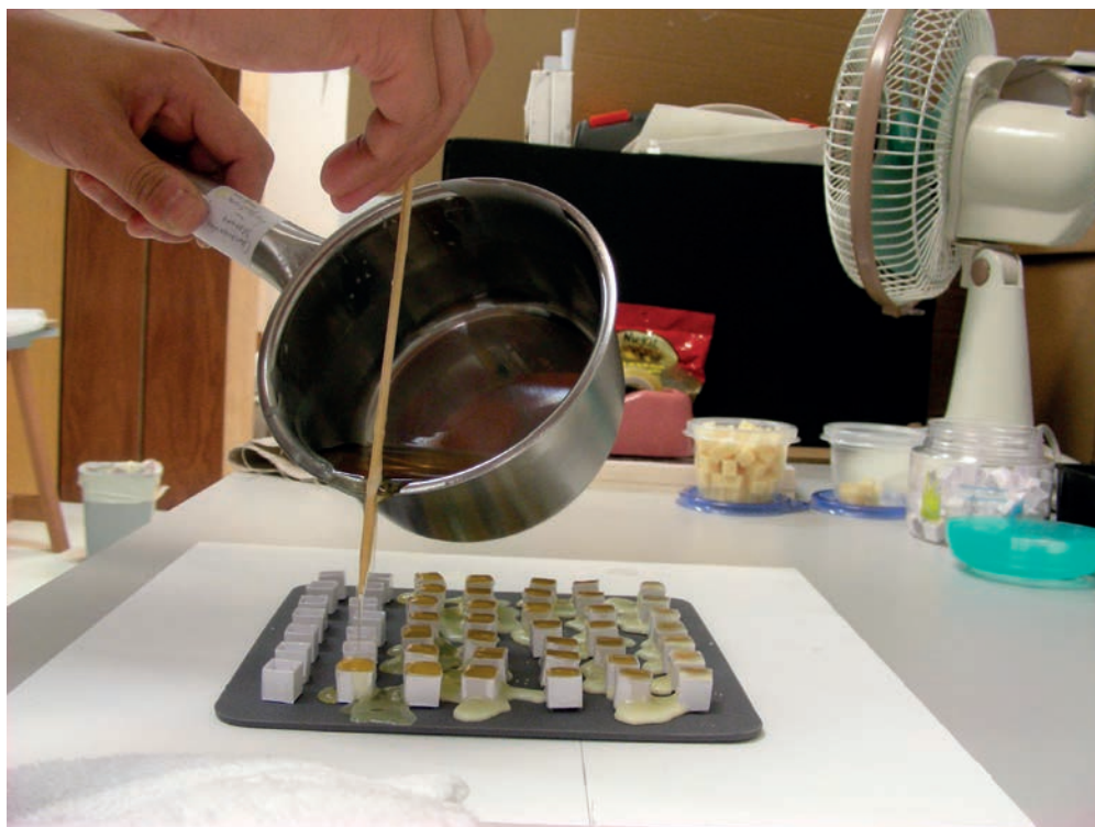
Figure 3 The production of the wax cubes used for embedding paint samples. (Photo: Claire Lim)
