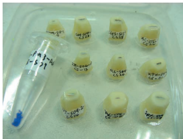
Figure 4 Paint samples embedded in wax (in readiness for microtoming for microscope observations and SEM-EDX). These are kept in plastic vials for future embedding and analysis. (Photo: Lawrence Chin)
